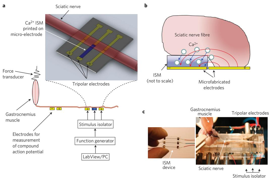
**Figure 1 | Principle and experimental set-up of functional electrochemical stimulation with *in situ* ion concentration modulation through ISMs.**
